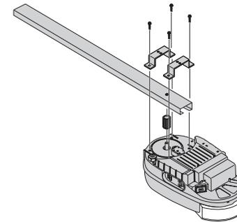
1. Install grey motorshaft adapter onto motorshaft. Bolt rail with brackets and screws to motorhousing. Make sure the screws are tightly fastened.
