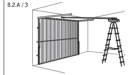
3. Disengage carriage from chain or belt!
