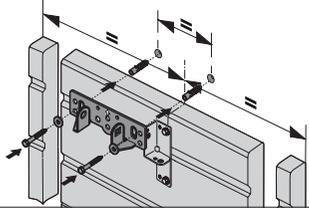
2. Install rail bracket on centre position above door. Make sure there is at least 10 mm clearance between highest travel point of door and rail.
