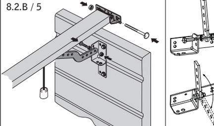
5. Connect operator pull bar to door bracket.
