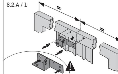
1. Install door bracket at centre position of door and rail bracket on centre position above door. Make sure there is at least 10 mm. clearance between highest travel point of door and rail.
