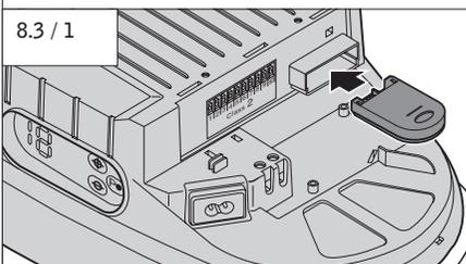
3. Insert the modular receiver in the opening of the operator. See fig. 8.3/1.
