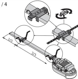
4. Disengage carriage from chain or belt. Door may only be moved with moderate speed.
