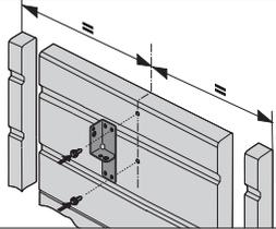
1. Fix adjustable door bracket to top section at the centre of the door.
