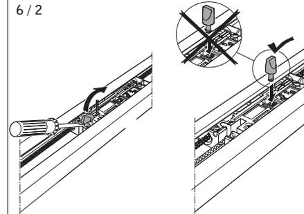
2. Fit the red slider that re-engages the emergency release and operator pull bar onto carriage.
